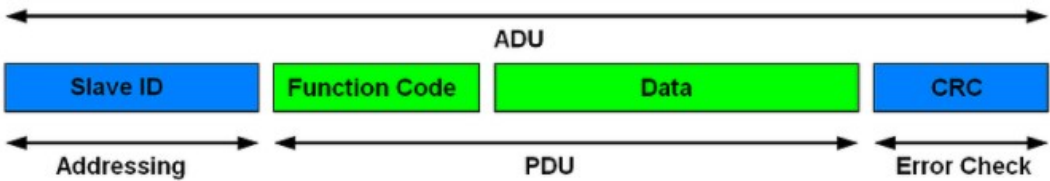
Fig. 107: Modbus/TCP and Modbus/RTU differences.
