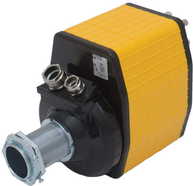
Slip ring collector consisting of rings coupled with brushes, designed to allow current to pass from a fixed to a rotating part and used to supply crane motors and cable winders.
